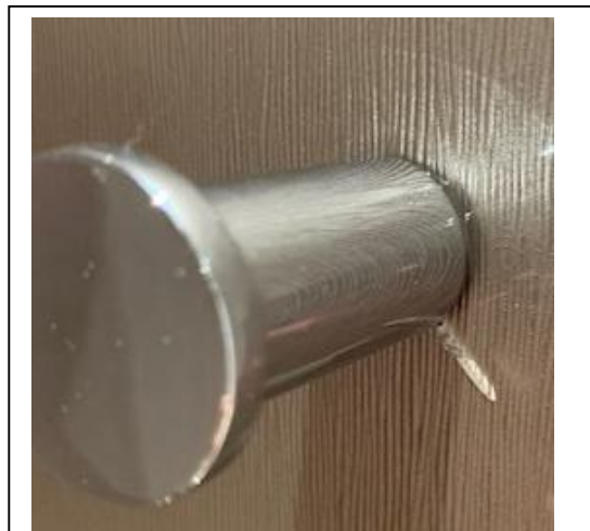
Fig 11 Example of excessive tightening
