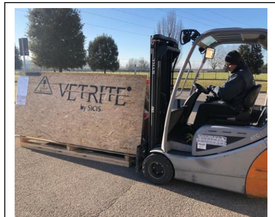
Fig 2 correct way of moving a VETRITE crate
